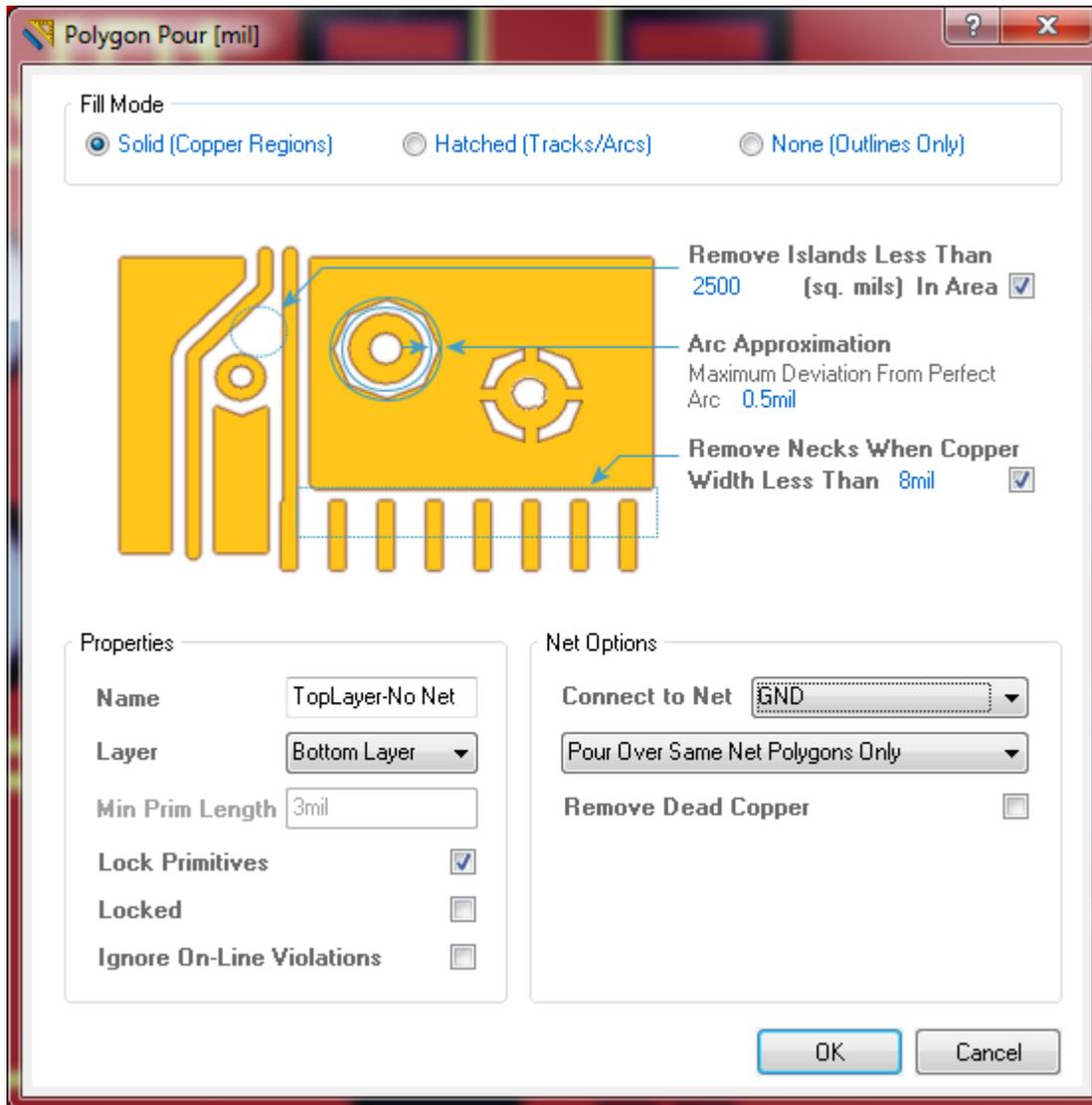
The bottom layer should be selected as well as the connection to the ground net.
