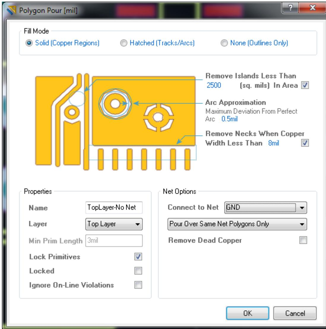
Set the layer to Top Layer and also set the “Connect to Net” to your ground net.
