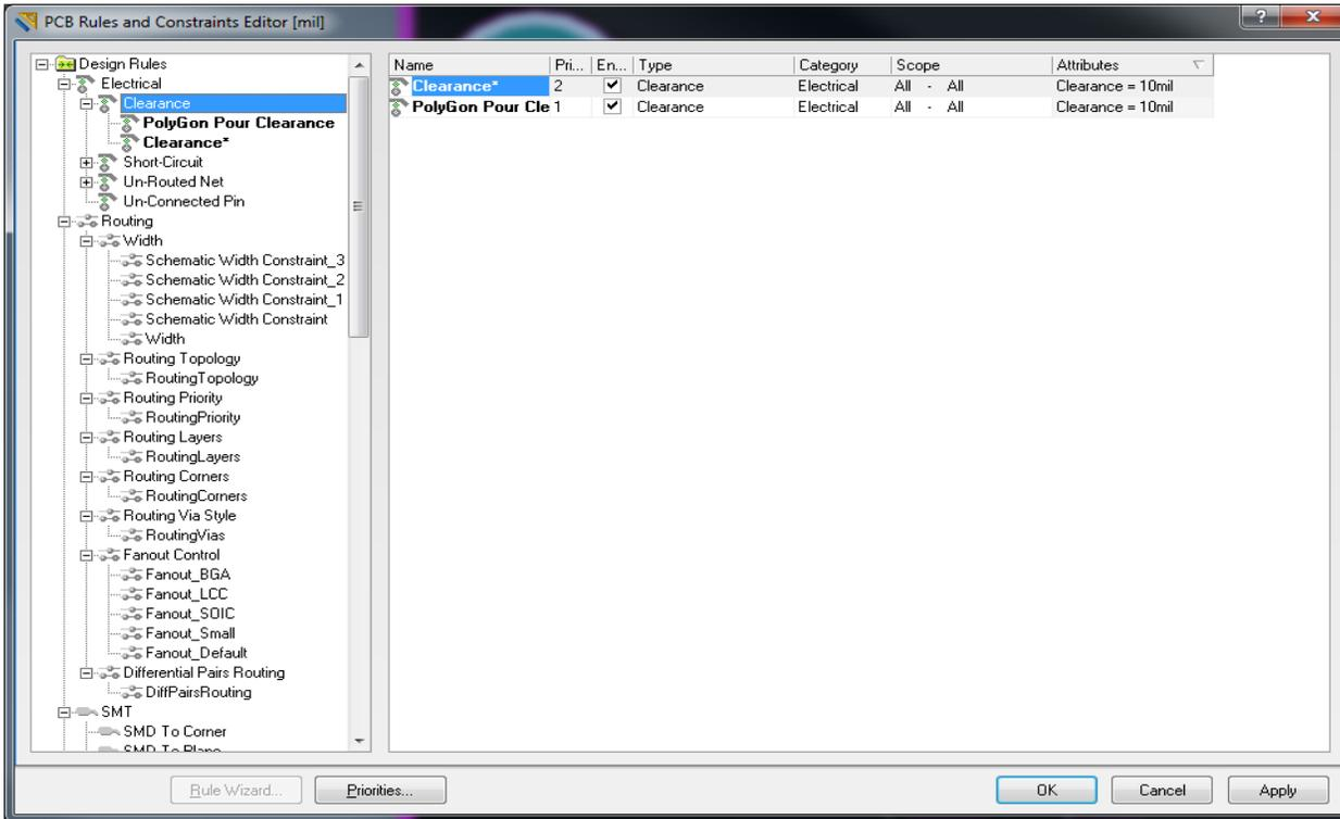
Click on the new rule on the left column. This will display the properties on the PolyGon Pour Clearance rule.
