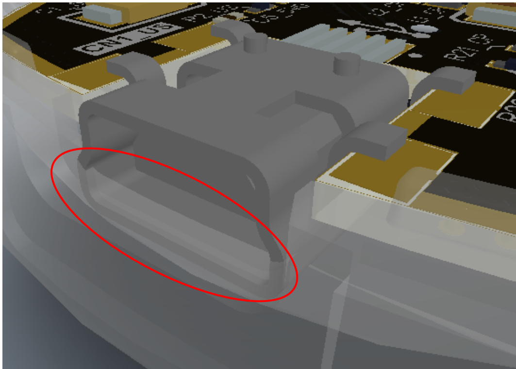
Figure 5. Note how connector is currently interfering with enclosure (DRC violations disabled).
